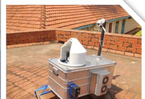
Wetland CH<sub>4</sub> emissions. First column measurement in East-Africa (in collaboration with Hartmut Bösch).
