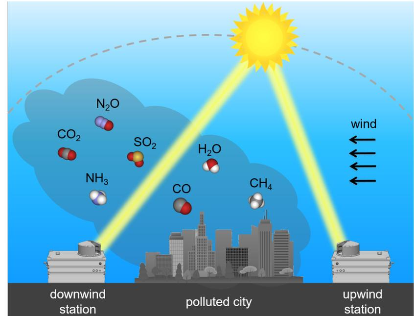
**Fig. 1:** Principle of the differential column measurements
