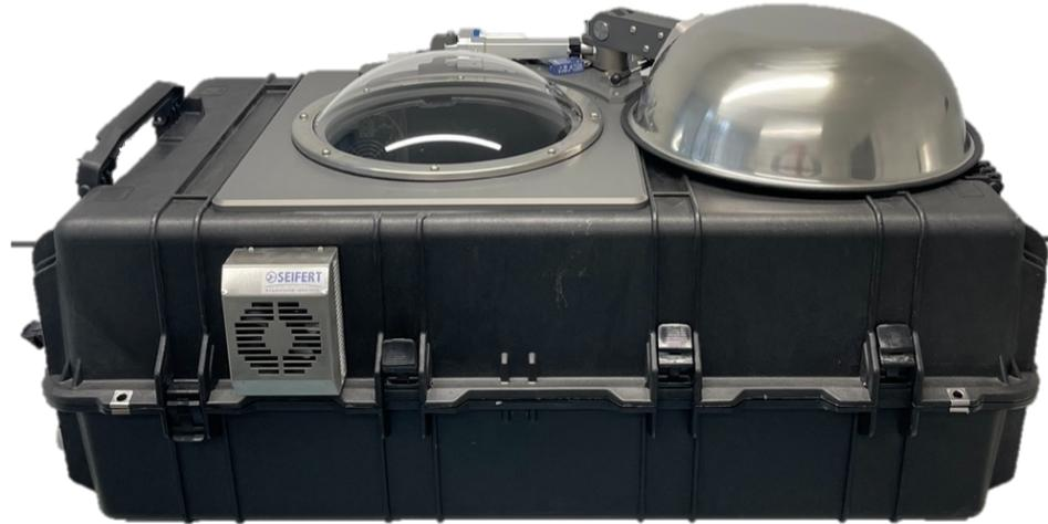
Fully enclosed (no air exchange), waterproof enclosure for EM27/SUN with precision optical dome with characterised transmission (BK7). Three enclosures previously deployed for > one year around London by NERC Field Spectroscopy Facility. Fourth enclosure deployed at RAL Space by University of Leicester. Ten more under construction as part of UK GHG monitoring network. Five more for University of Edinburgh.
