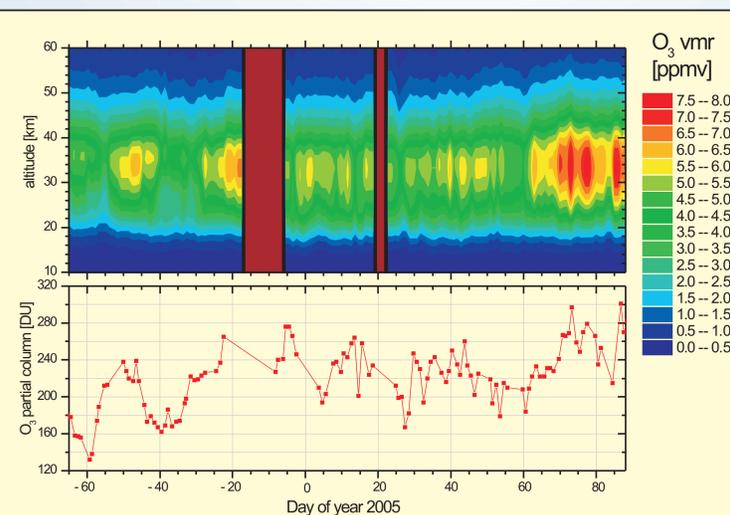
**Figure 2:** Time series of ozone during winter/spring 2004/05 (upper panel). The contour plot shows the volume mixing ratio in ppmv. The lower panel presents the partial ozone column density from 10 to 60 km.
