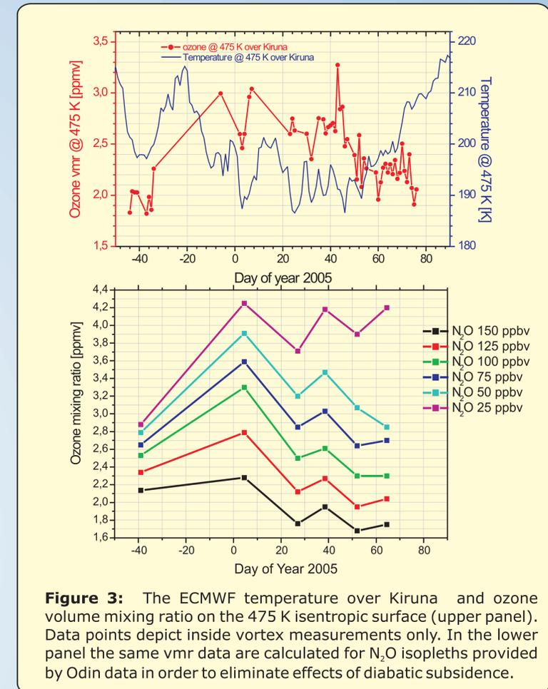
**Figure 3:** The ECMWF temperature over Kiruna and ozone volume mixing ratio on the 475 K isentropic surface (upper panel). Data points depict inside vortex measurements only. In the lower panel the same vmr data are calculated for N<sub>2</sub>O isopleths provided by Odin data in order to eliminate effects of diabatic subsidence.
