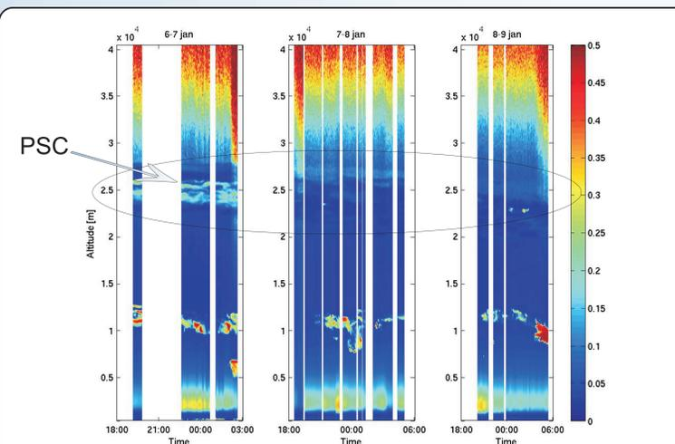
**Figure 5:** Observations of the new IRF lidar system from Jan 6-9. The layer at around 10 km depicts high cirrus clouds. The layer at 25 km indicates PSC (type II) with moderate depolarization on Jan 7. PSC with low depolarization (type I) were observed Jan 8-9.
