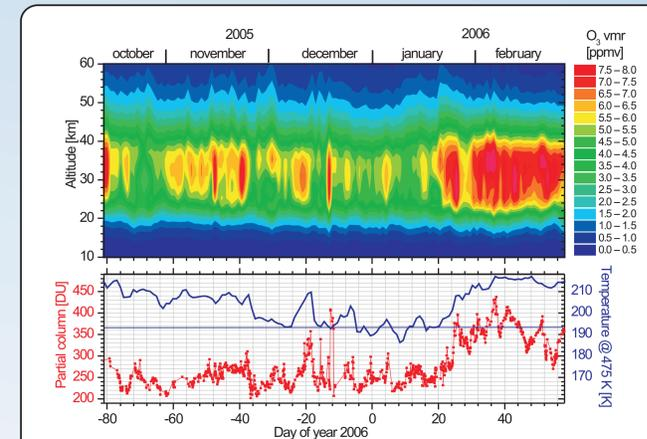
**Figure 2:** Time series of O<sub>3</sub> during winter 2005/06 (upper panel). The contour plot shows the volume mixing ratio in ppmv. The lower panel presents the partial O<sub>3</sub> column density from 10 to 80 km. The blue line indicates the temperature at 475 K isentropic level over Kiruna.
